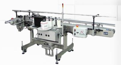
This labeling system features our heavy-duty printer applicator and a secondary pneumatic cylinder impresser.
