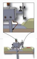
The Q.A.scanner can be affixed in several places after the tag or label is applied, but is normally right after the application device. Close detection allows you time to perform reaction tasks such as stopping the line, or auto reject. Low light and dusty environments are not an issue for the device, and is a 7/24 rated device.
