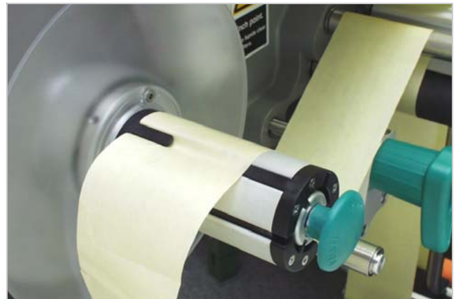
[45] Fastening the backing paper to the rewinder.
