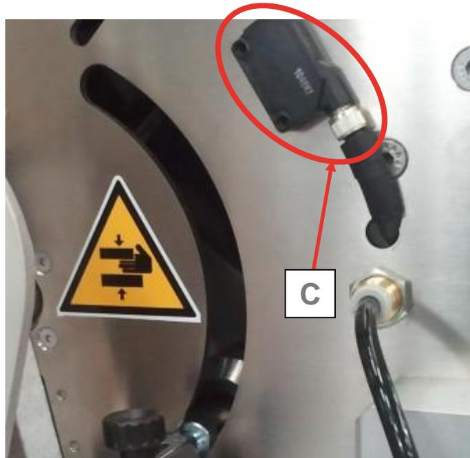
(Fig. 2.5.3 – Label detection photocell)
