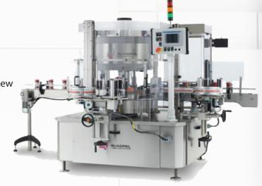
Additional features include Allen-Bradley® PLC, PanelView® color touchscreen, servo driven label feed and internationally compliant guarding. This labeling system combines world class product handling with technically advanced controls creating a product decoration system unsurpassed in accuracy, reliability and performance.
