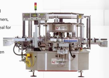
This system is designed to accommodate up to four label applicators and is capable of applying front/back, wraparound, neck and spot labels at up to 350 products per minute. It may also be configured to automatically switch from one applicator to another for nonstop, zero-downtime production.
